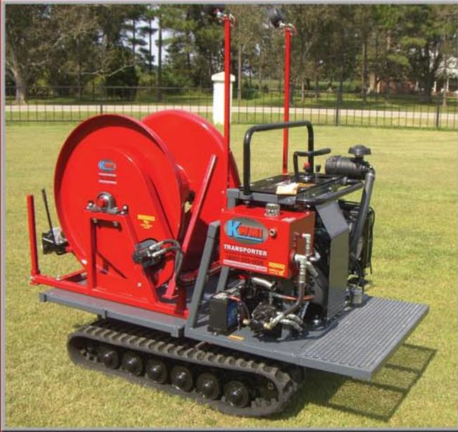
The KWMI Easement Machine is an all-terrain rubber tracked power carrier designed specifically for the pumper-cleaner industry.
