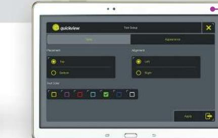
**Text Overlay.** Configure on-screen display of text, including variables like zoom, tilt and GPS coordinates. Modify text color and position.
