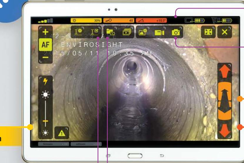
**Status Bar.** Monitor illumination, zoom and tilt, as well as Wi-Fi signal and battery (for both tablet and camera).
