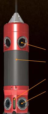
Four laser scanners generate a dense point cloud for 3D analysis.
